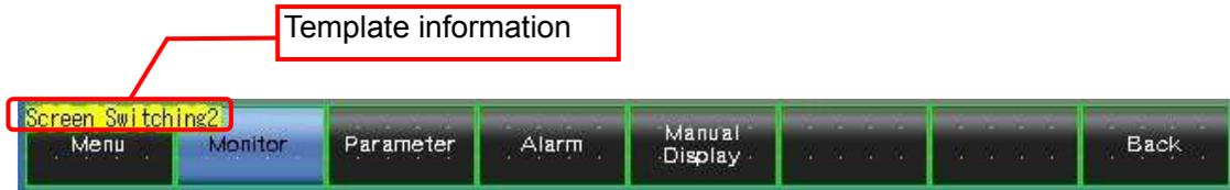
The template information is only displayed on the screen design software's editing screen. It is not displayed on the GOT display screen.
