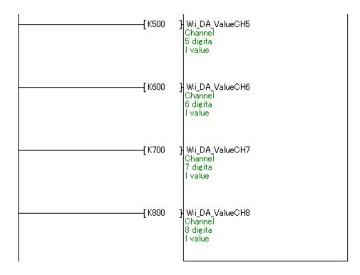
M+Q68DA\_SetDAConversion (DA conversion enable/disable setting)
