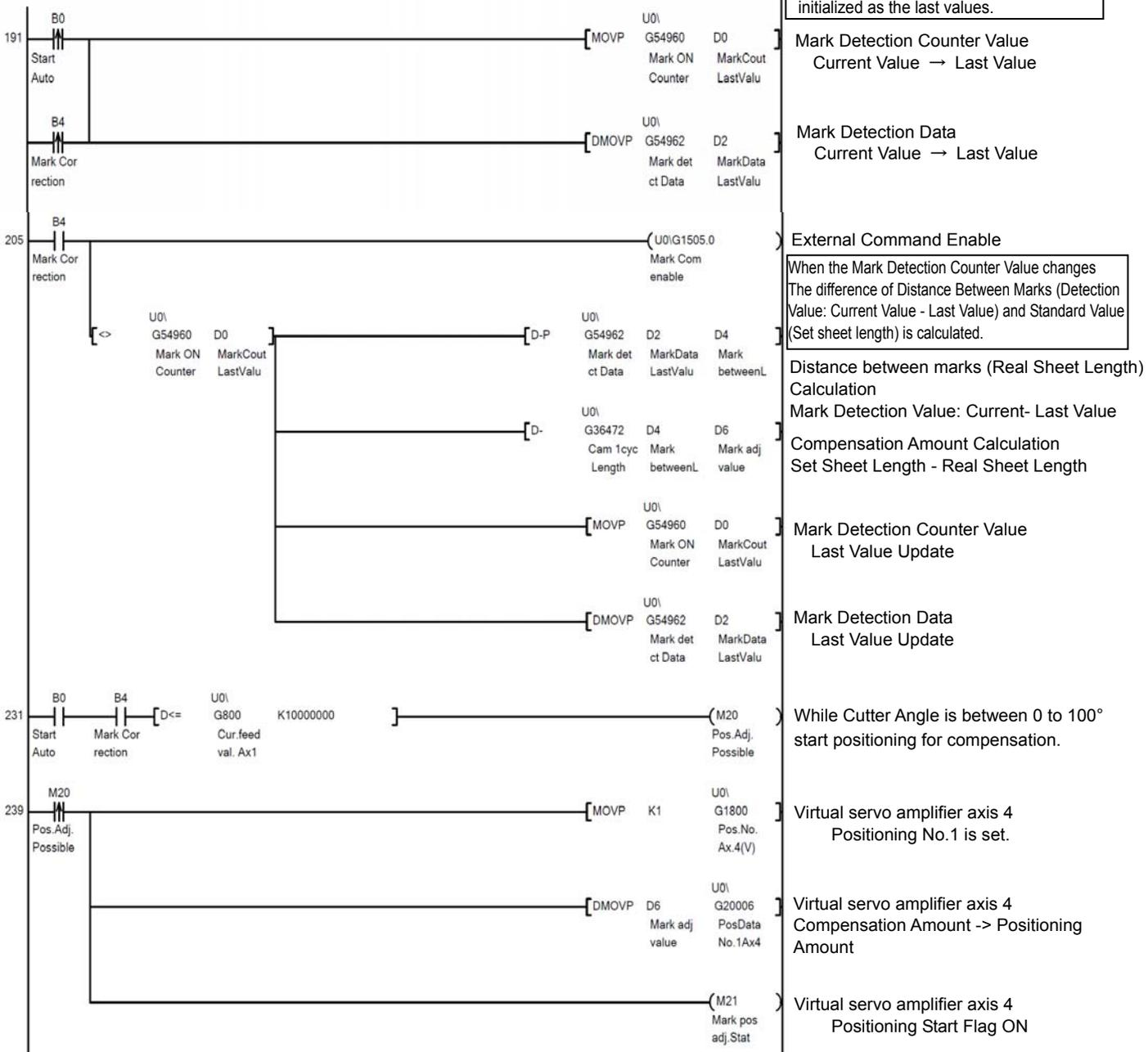
When Automatic Operation Starts or Mark Compensation is started the values are initialized as the last values.
