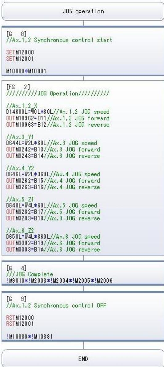
X-Axis (Axis 1, 2) Synchronous Control Start
